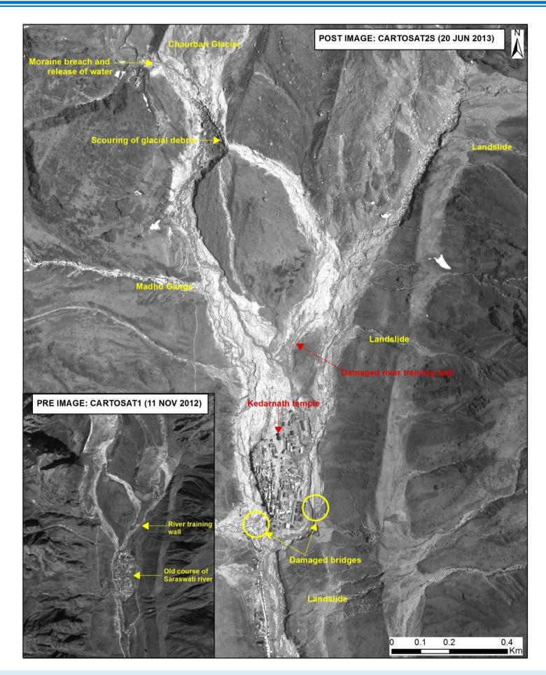
Figure 6. Geomorphological changes leading to the disaster around Kedarnath, Uttarakhand (2013). Satellite data
